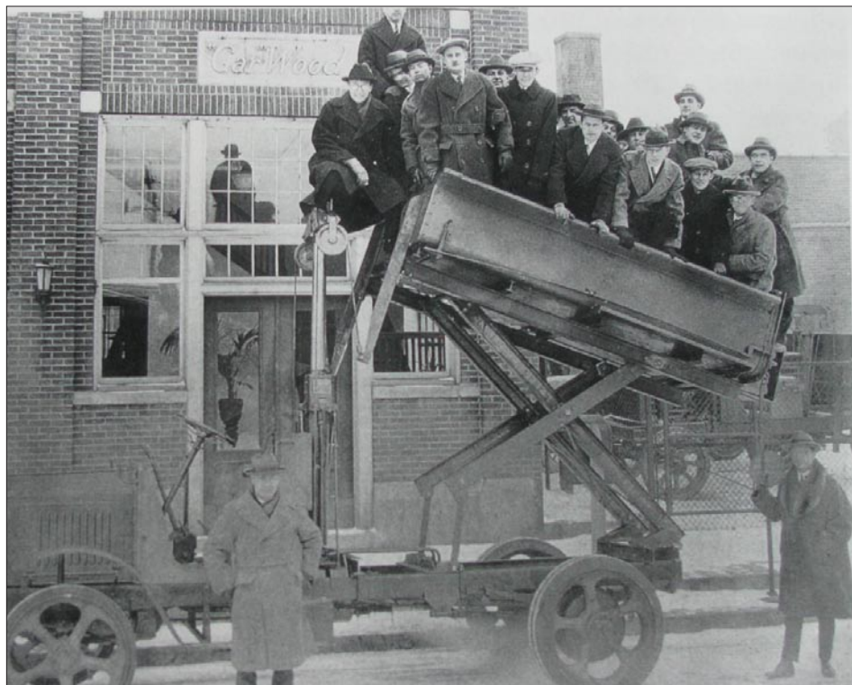
With 18 men in the cargo bed, this truck demonstrates the lifting power of Wood's patented hydraulic hoist which would eventually be used in dump trucks around the world, making Gar Wood and his wife millionaires.
